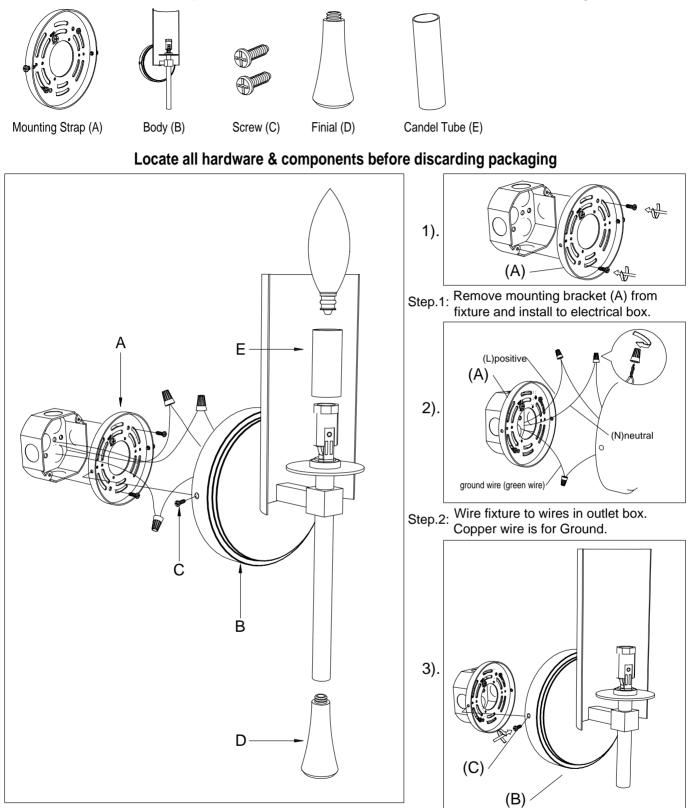
Step.3: Install body (B) to the outlet box and secure with screw(C). Install finial (D) on the body. Place the Candle Tube (E) over the socket, Install light bulb.
